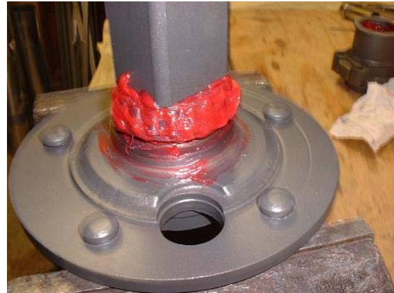
22. Be sure to put the bearing on the axle shaft in the right direction. Drive it down until it seats on the bottom.
