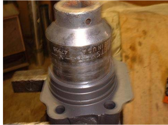
18. After cleaning all the parts start the reassembly by driving in the bearing cups. Use drivers or a socket that fits the outer edge of the cup.
