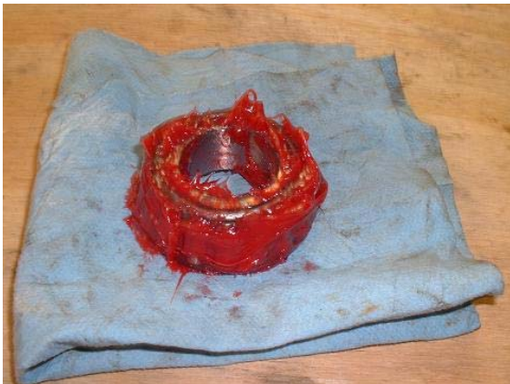
21. Pack all the bearings at once to facilitate clean up. Smear grease on the outside of the bearing and anywhere the packer didn't fill.
