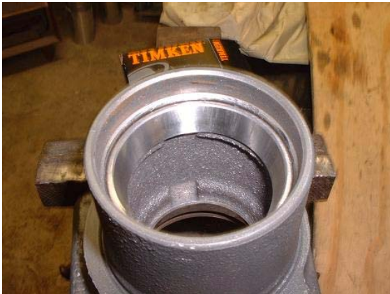
19. Drive the bearing cup all the way down until it contacts the bottom of the flange. Now flip the hub over and install the other bearing cup.
