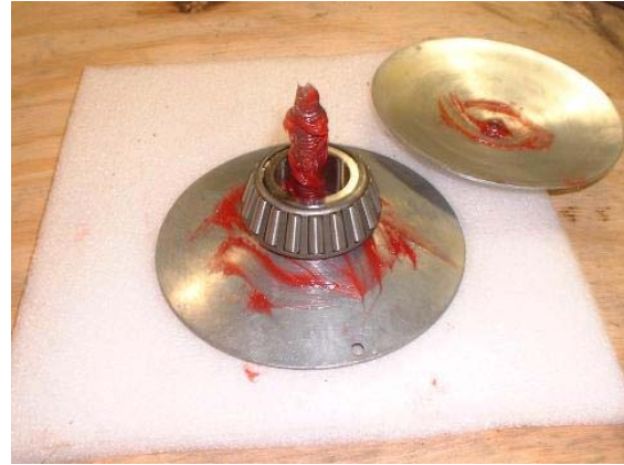
20. Here is one tool I recommend every DIYer own. A bearing packer uses a grease gun to force grease into the bearing much easier than by hand.
